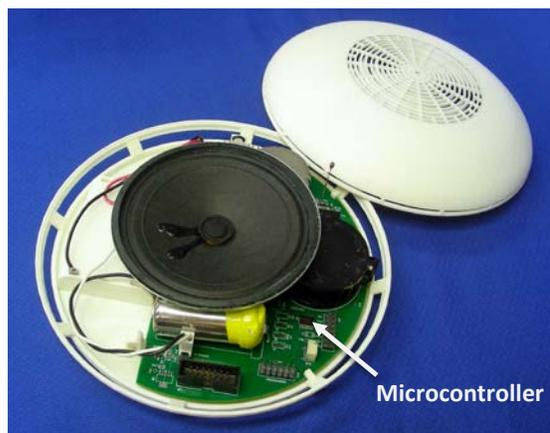
Figure 1. Assembled prototype incorporating multiple sensors, a microcontroller, power (3 AA batteries), and a speaker for 520Hz alerting. The enclosure is 6.5" in diameter and 1.7" tall.
